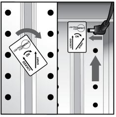
**3C:** The LED cord will include three (3) built-in clips to attache and manage the cord placement. Utilize these to secure the cord to the underside of shelf. If needed, the clips can be slid on the cord to reposition. This process will help keep the cord up and away from the product, shoppers, and staff.
