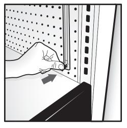
[Optional] — 1C: A containment strap has been provided if additional support is needed in the center of the power strip. Align the two pegs on the back of the strap with holes in the peg board, and push in place until it's flush with power strip.
