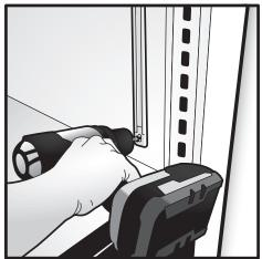
[Optional] — 1C: Screw guides have been provided if additional support is needed in the center of the power strip. Snap the screw guide onto power strip in the desired location.
