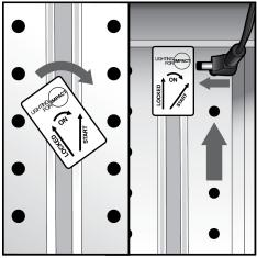
**3C:** Use the plastic "twist" clips to secure the LED cord to the wire shelving. Two clips are provided per shelf. First, insert the LED cord into a clip. Then, align clip with a wire on the shelf and twist to lock in place. These clips will help keep the cord up and away from the product.
